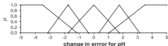
Fig. 12. Fuzzy membership function for a change in error for pH (for the set points of positive and negative effects).
